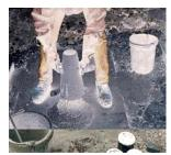
It is a concrete mixture that can be placed purely by means of its own weight with little or no vibration. Adjustments to traditional mix design and the use of superplasticizers creates flowing concrete that meets performance requirements. SCC's unique properties give it significant economic, constructability, aes-
