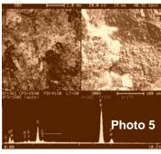
The analysis of the corrosion deposits on the outside of the pipe by Energy Dispersive X-ray (EDX) showed a high concentration of sulfur in addition to smaller amounts of chlorine. Photo 6 is a typical EDX spectrum representing all the elements found.
