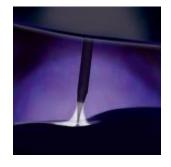
method of GMAW is the reduction in spatter over that of the steady current short-circuit method.
