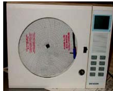
Curing Room Thermometer
